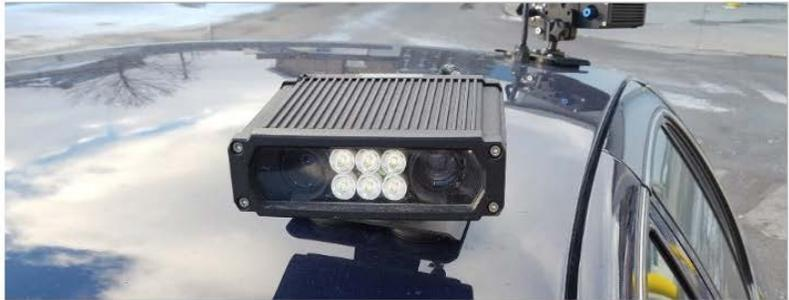
Our Service uses the Automated Licence Plate Recognition System (ALPRS), which is installed on a police cruiser and used to automatically scan licence plates up to 20 metres away. The system will alert our officers of stolen plates and vehicles, plates registered to suspended drivers, expired permits and other offences.
