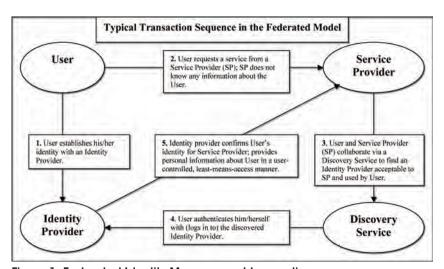
Figure 1: Federated Identity Management transaction sequence
